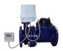
In order to solve the problem of difficult charging for water supply departments in most areas at home and abroad, this product was developed. Its biggest feature is to pay first, then use water. When the balance in the water meter is zero, the valve automatically closes until the user completes the recharge again.
